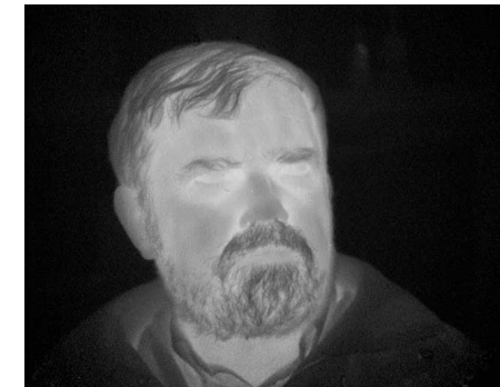
Courtesy of 8.6 \mu\text{m} thermal image taken with large format 640x512 QWIP FPA IntelliEPI. Die size \sim 16 \times 13 \text{ mm}^2 .
